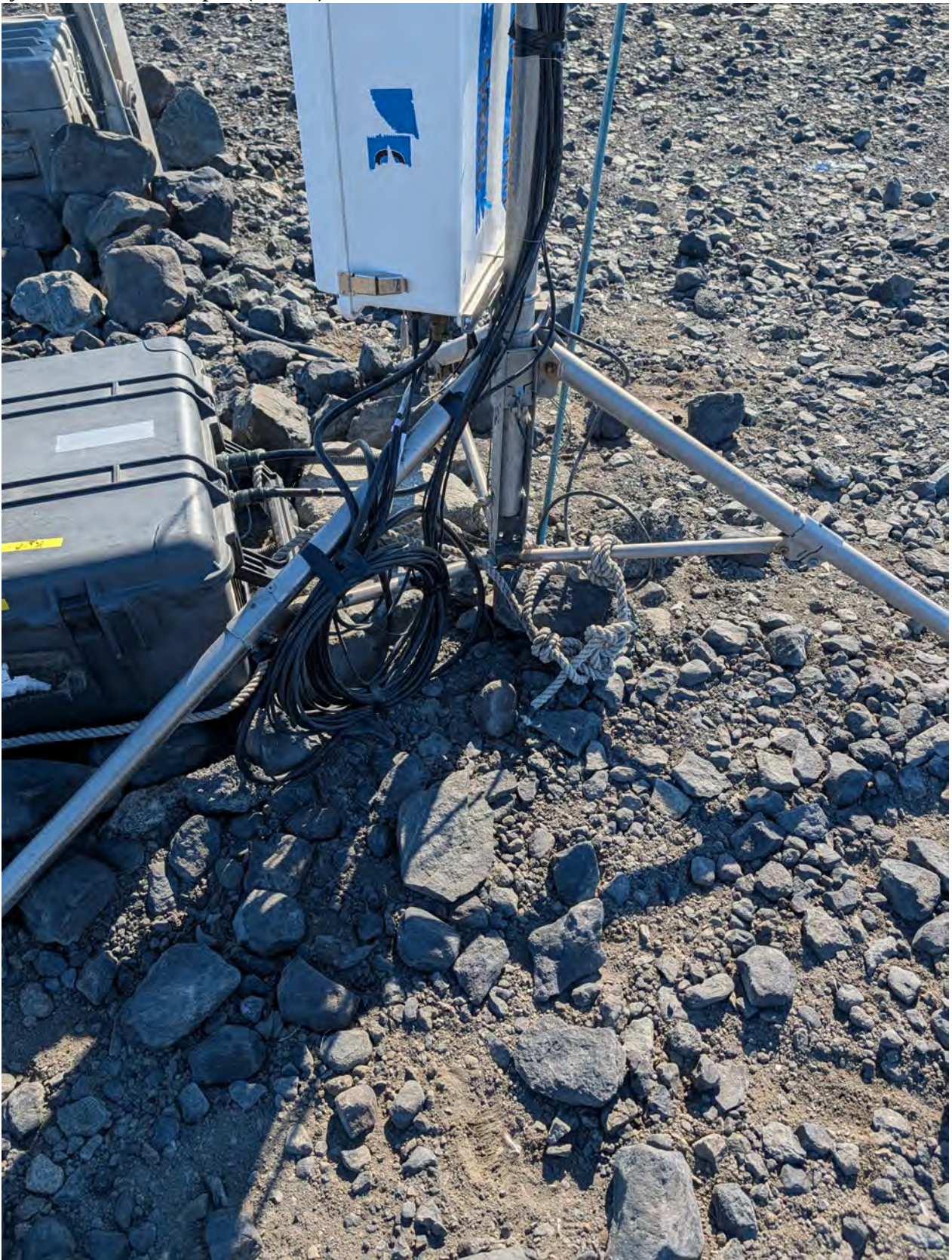
Battery box fastened to tripod (view 2)
