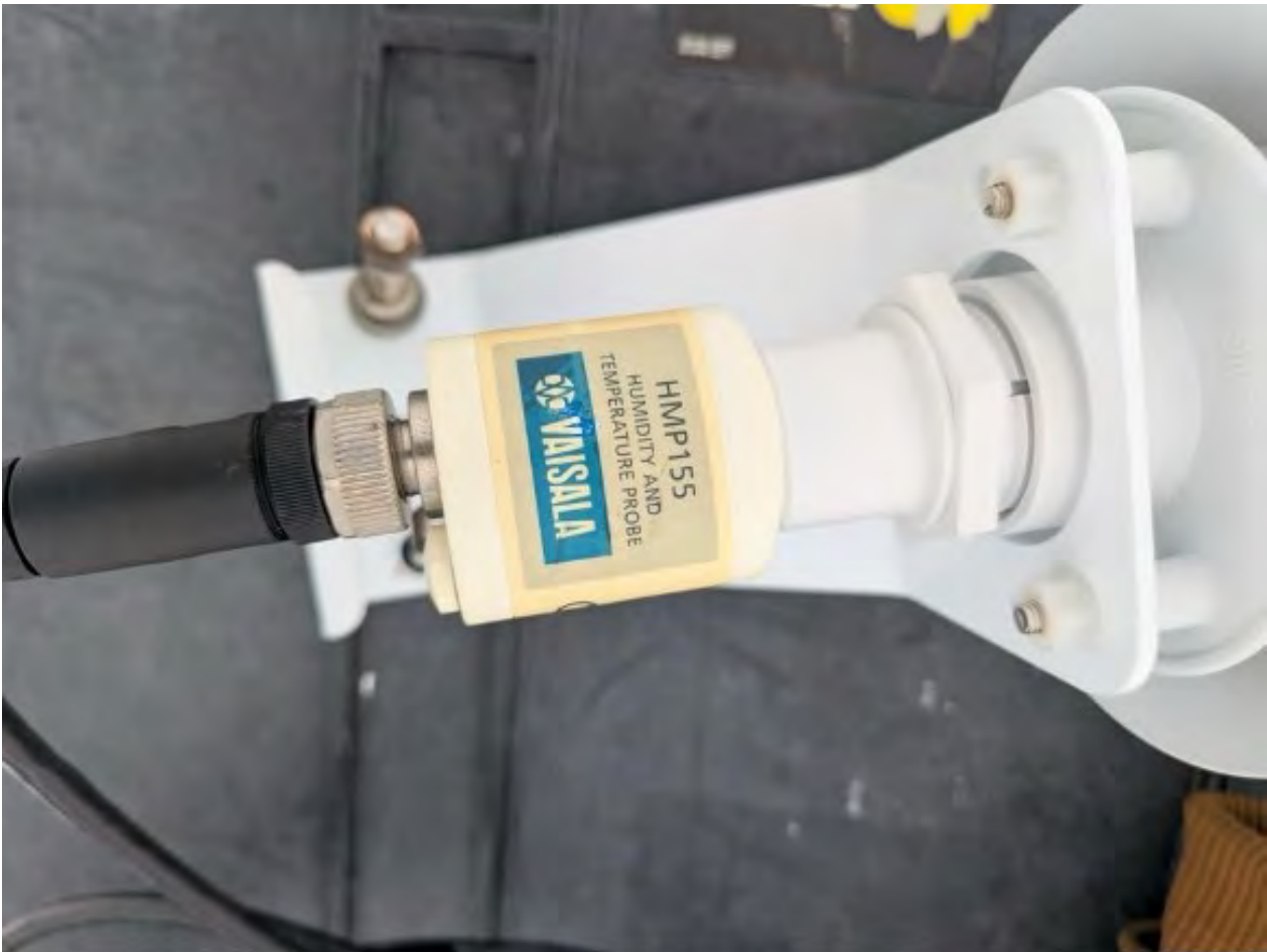
RH sensor that was removed
