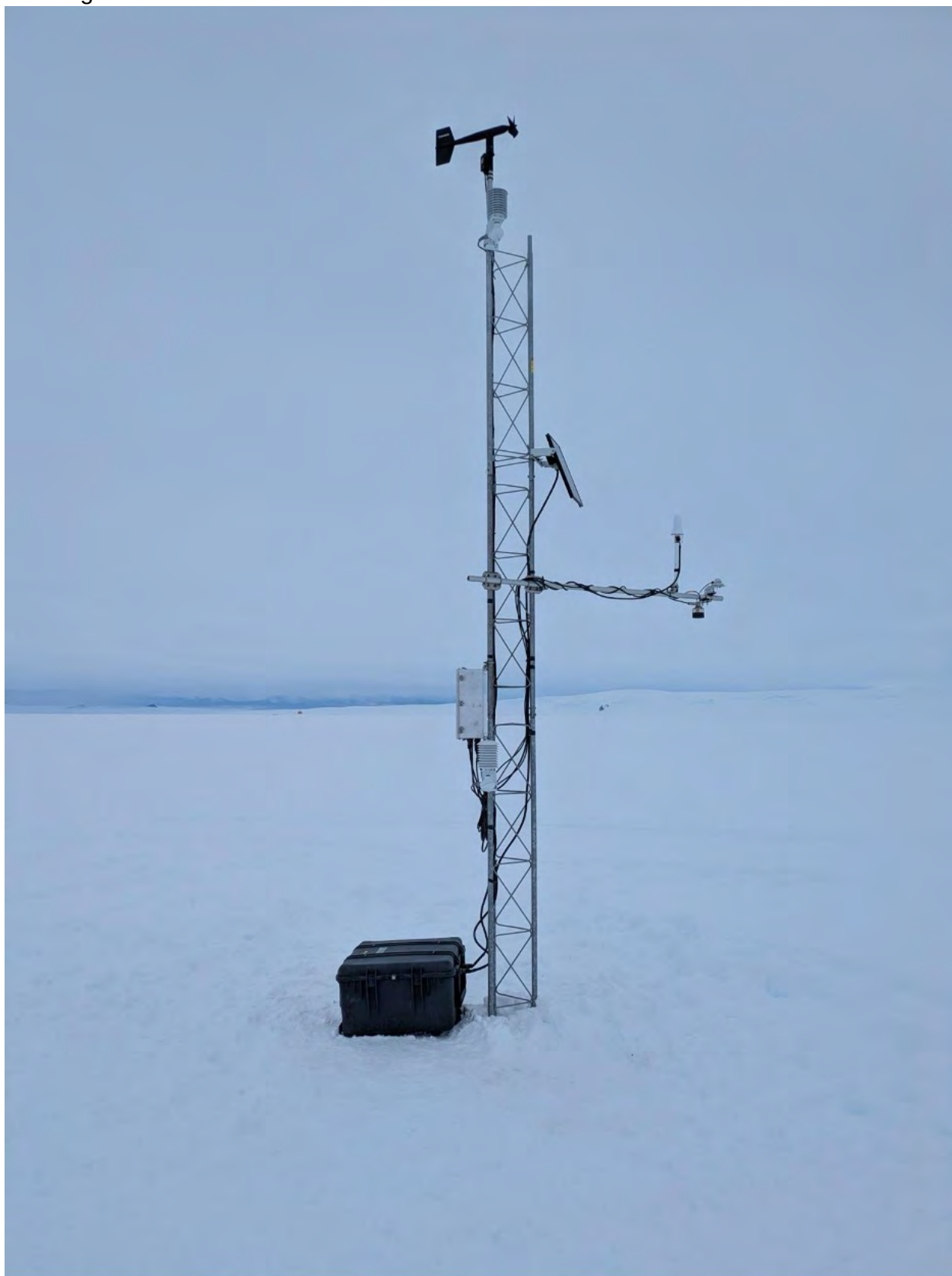
Windless Bight AWS after RH sensor was removed.
